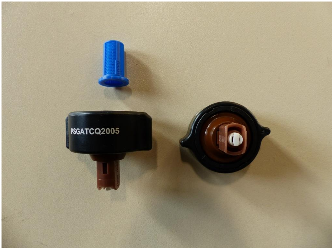
Double - Flatfan nozzle John Deere PSGATCQ2005 (ceramics, plastic-coated, brown)
